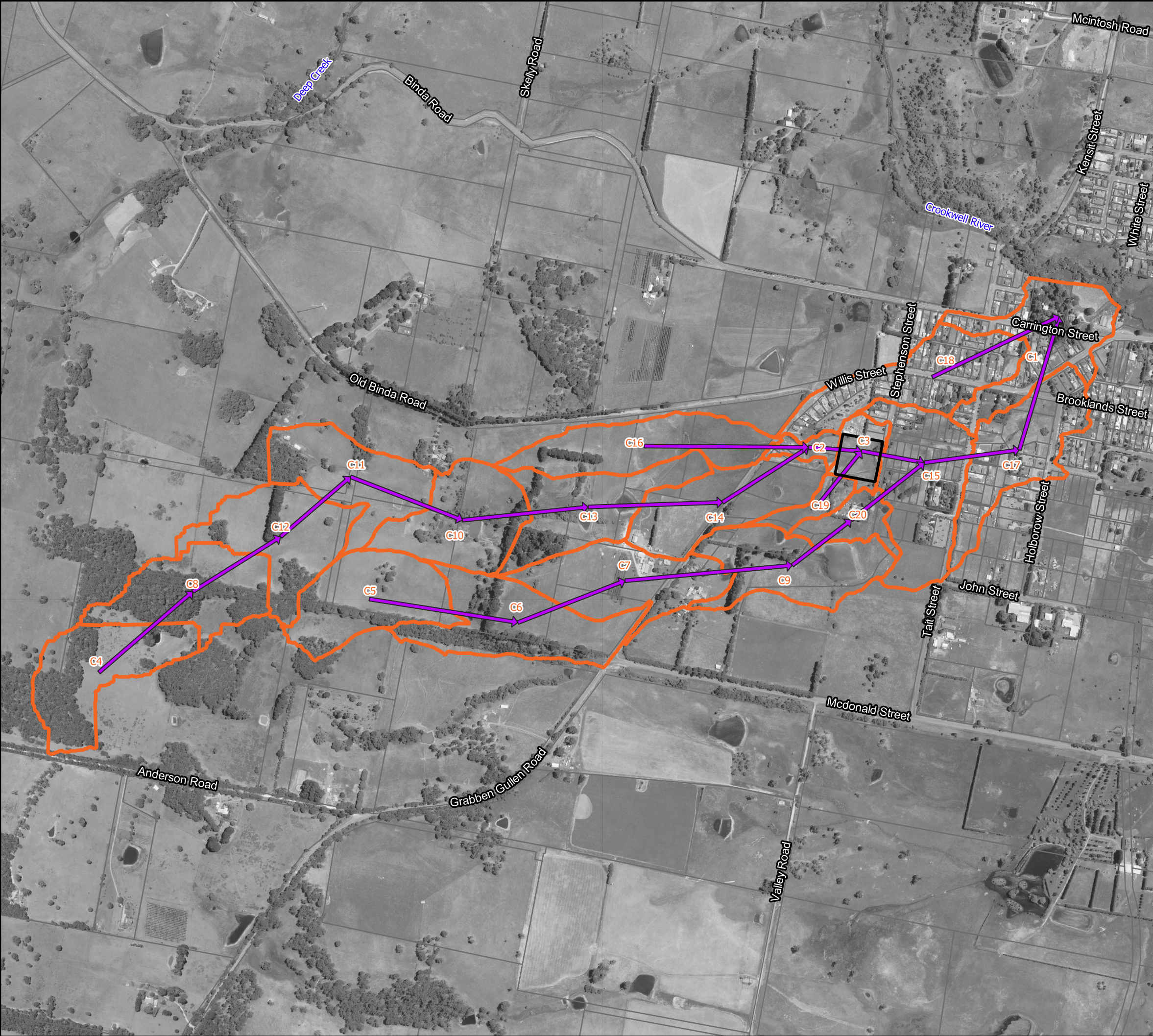
Figure 2: XP-RAFTS Subcatchment Layout
