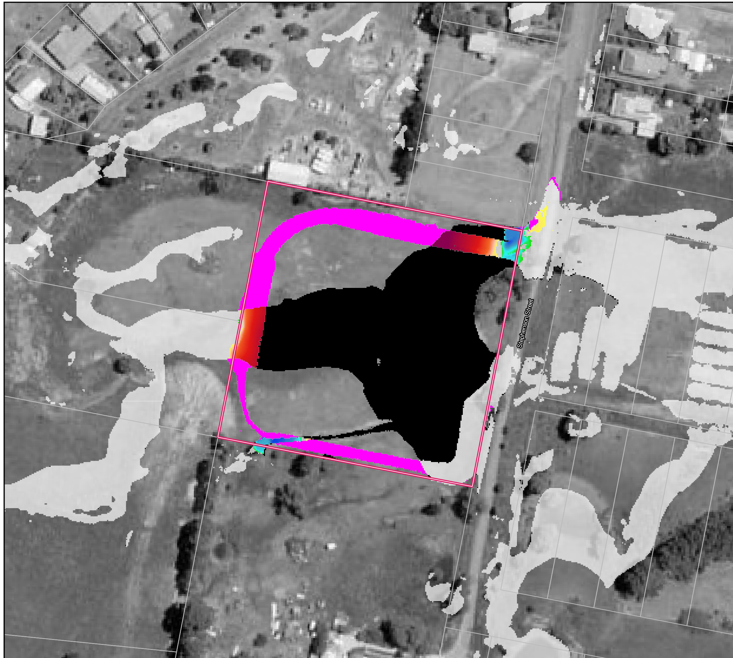
Figure 13: Predicted Change in Peak 1% AEP Flood Levels with Climate Change
